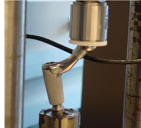
Taper junction fatigue testing 1,2
