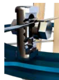
FIGURE 17 Wire Post in final position to capture the Wire.
