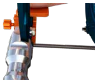
FIGURE 29 This illustration shows the Tensioner seated properly over the Ring and the Wire Bolt.
