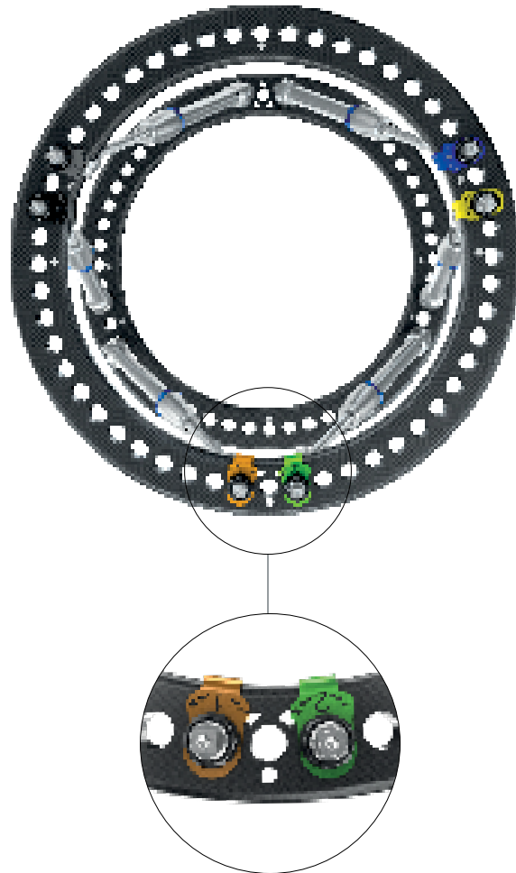
Nominal strut mounting sites: full ring (reference ring).
