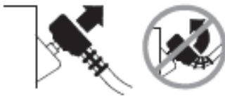
Figure 5-5 Disconnecting Defibrillation Cable from Test Post
