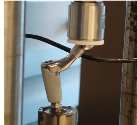
Taper junction fatigue testing 1,2
