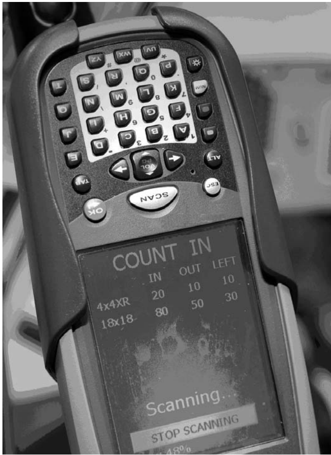
Figure 2. The data-matrix scanner shows the type of and the number of sponges still on the sterile field and the number of sponges that have been removed from the sterile field. (Figure 2 is available in color in online article.)
