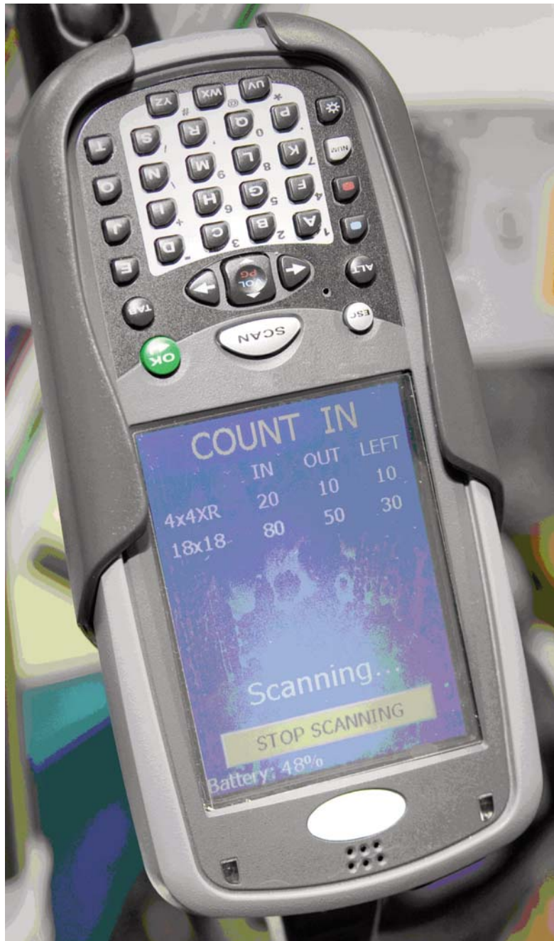
Figure 2. The data-matrix scanner shows the type of and the number of sponges still on the sterile field and the number of sponges that have been removed from the sterile field.
